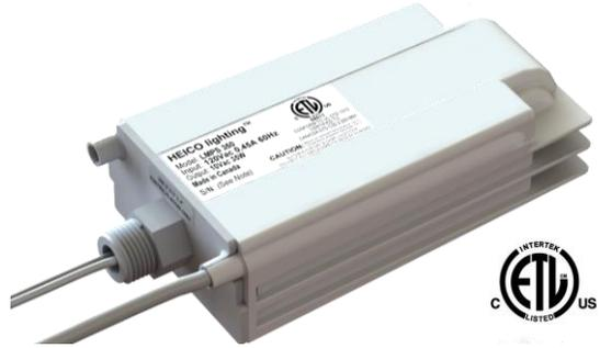
Designed for the architectural lighting industry, the **LMPS-350** power supply is part of the **HEICO lighting™ Contactless LED System**. The power supply is fully potted and suitable for use in dry and damp locations. The AC power of the LMPS is fed by electromagnetic induction to the LED array, which eliminates electrical contacts and risks of corrosion. The LMPS-350 is UL 1310 and its output is compliant to Class 2 security extra low voltage (SELV).
